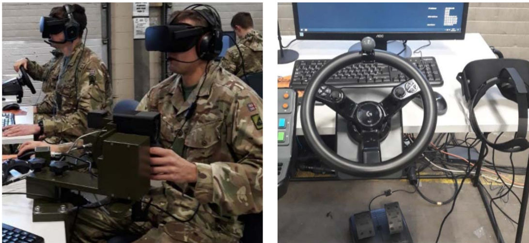
Figure 4-2: Warrior High Fidelity Gunner Controller with Trainee Using VR HMD (L) and Warrior Driver COTS Steering Wheel and Accelerator and Brake Foot Pedals (R)
